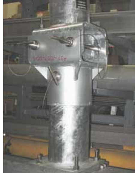
SM-DVT-PA: Davit portable adapter is slipped over the stanchion davit pedestal base and then attached to the davit socket.
